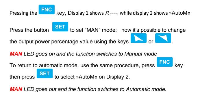
If the sensor breaks during Automatic functioning, controller moves to Manual mode while maintaining the output percentage command unchanged as generated by the PID immediately before breakage. If there is a temporary power failure or after switch-off ,manual functioning as well as the previous output percentage value will be maintained at restarting
