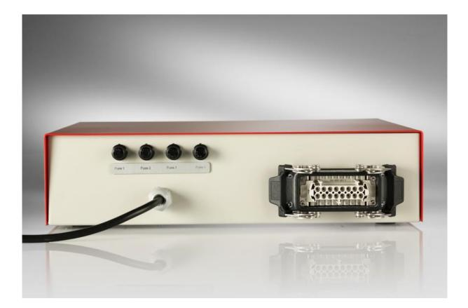
24 pin ILME Connector CNEF 24 / CHI 24 Thermocouple type J / K
