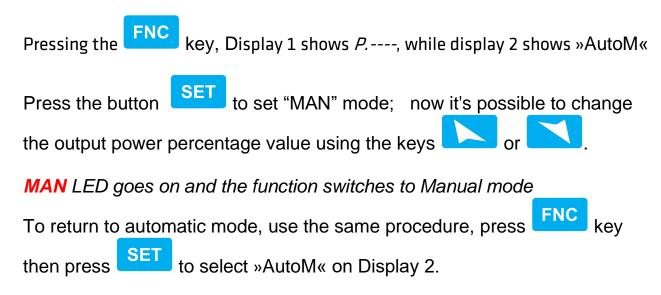
MAN LED goes out and the function switches to Automatic mode.
